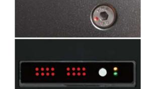
housing, there are two hex screws and a small hole with a pin inside it, indicating the vertical position of the upper plate for balancing purpose.
