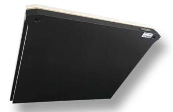
The upper and lower surfaces of the Silence Plus are separated by a permanently elastic gel. This THIXAR-typical material has the effect of inhibiting the transmission of signals from top to bottom and vice versa. Additional materials are embedded in this special gel that selectively absorb medium-frequency vibrations and eliminate them in combination with the gel.
